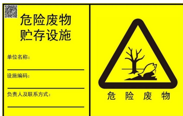
图 4-7 危废仓库室外危险废物标签
